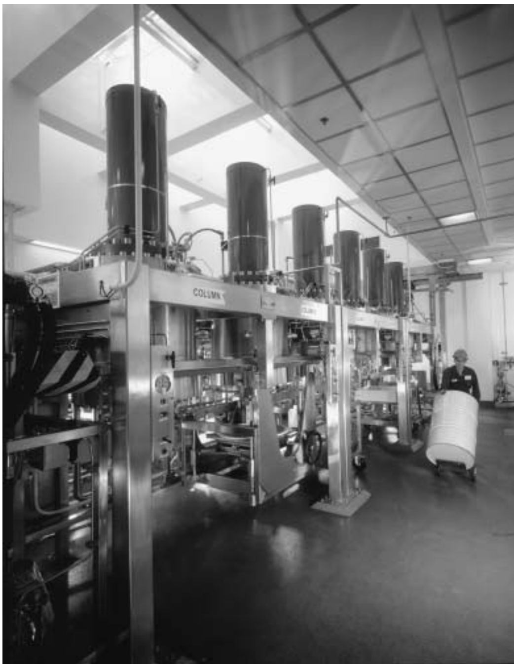
Figure 11.2 Multicolumn continuous chromatography unit (MCC 6×800) used for the separation of an API at commercial scale. Photograph courtesy of Aerojet Fine Chemicals, Sacramento, CA.
