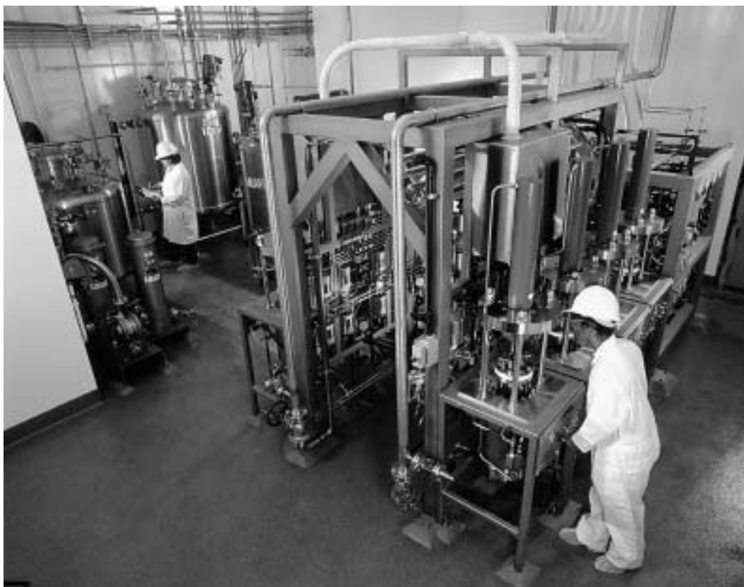
Figure 11.1 Multicolumn continuous chromatography equipment (MCC 8 × 200) used for purification of material for clinical trial. Photography courtesy of Aerojet Fine Chemicals, Sacramento, CA.
