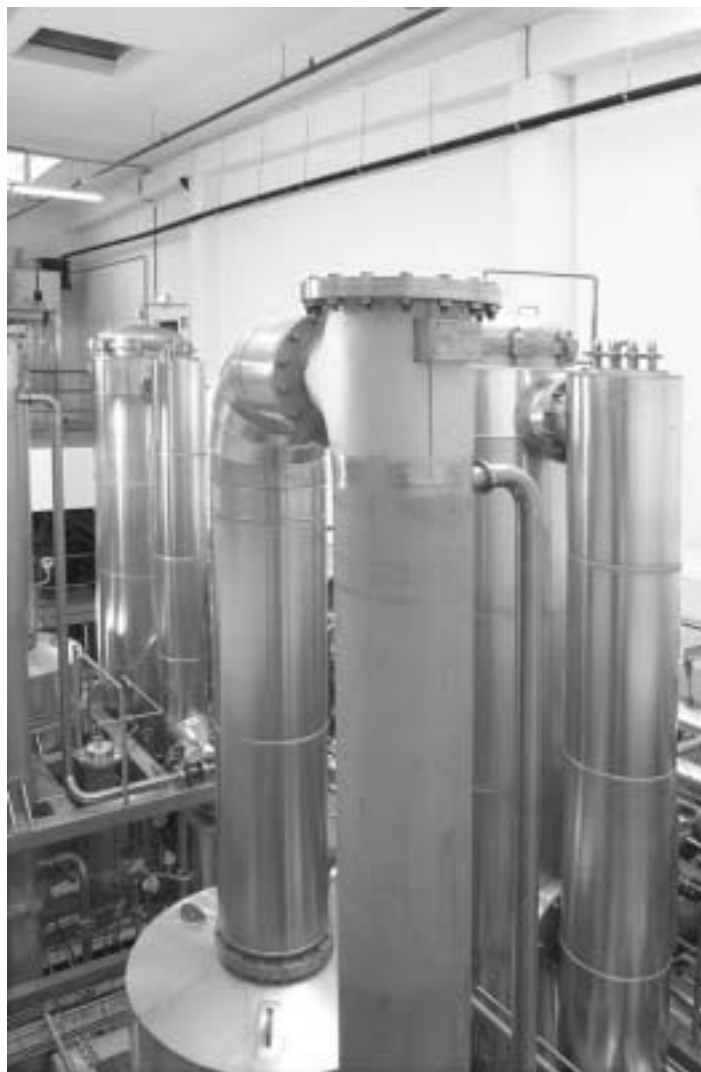
Figure 10.16 Falling film evaporators used for solvent recovery in an MCC 5-1000 unit at UCB Pharma (Braine, Belgium).
