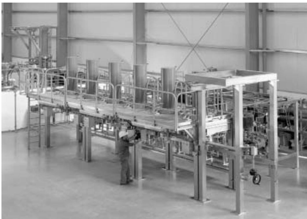
Figure 9.13 VARICOL unit equipped for five columns of 1000 mm i.d. Courtesy of NOVASEP.
